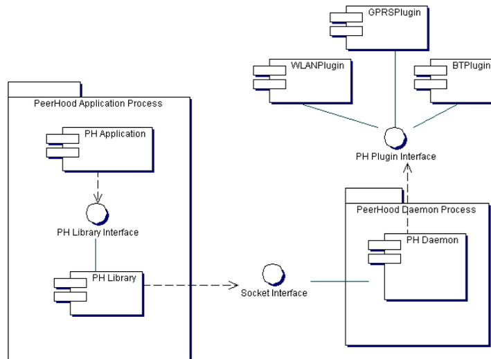
Figure 5. Components of the Linux PeerHood
