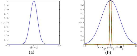
Fig. 3. Likelihoods for: (a) Measurement model,  $p(d|d^*)$ ; (b) Grasp stability,  $P(S|G, O)$ , for  $(x, y, \theta)$ ,  $x$  in red,  $y$  in dashed green,  $\theta$  in blue.
