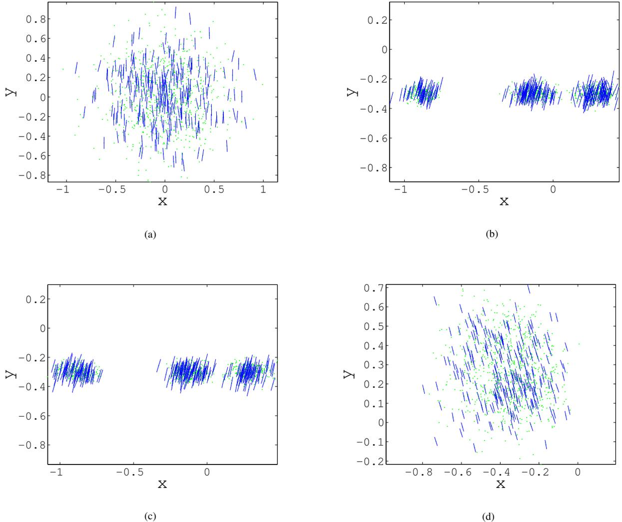
Fig. 4. Sequential distributions of particles modeling  $P(O|G, T)$ , (a)-(c), for a single run of Algorithm 1: (a) Initial distribution ; (b) Distribution after the first grasp; (c) Distribution after second grasp, for which  $P(S|G, O) = 0.503$ ; (d) An example of distribution  $P(S|G, O)$
